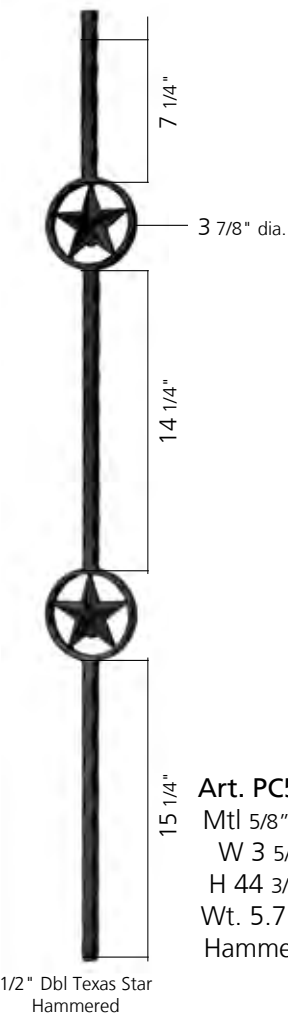
Art. PC26/1 Mtl 1/2" sq. W 7 1/2" H 44 3/32" Wt. 6.9 lbs Hammered
