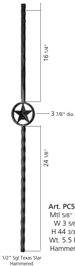
Art. PC33/1 Mtl 1/2" sq. W 5 5/16" H 44 3/32" Wt. 5.5 lbs. Hammered
